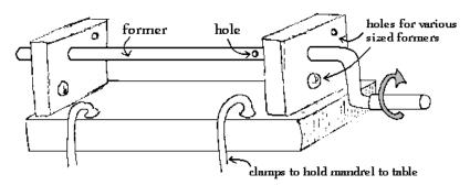
and efficiently. The Jig would have a slot or hole to hold one end of the wire while it was wound under tension.
